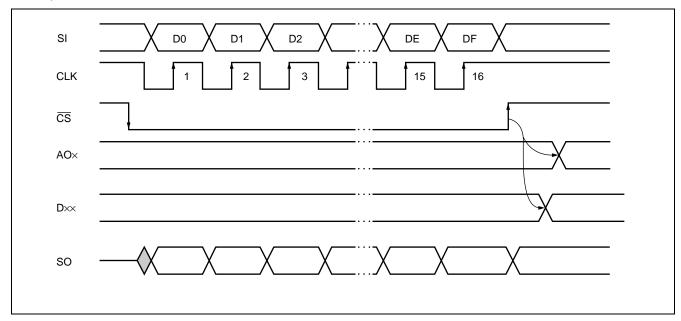
Data input is enabled at the fall of the  $\overline{CS}$  signal. 16-bit data is input, and executed by shift register command at the rise of  $\overline{CS}$ .
