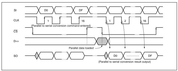
Data input is enabled at the fall of the  $\overline{CS}$  signal. 16-bit data (parallel to serial conversion command) is input, and commands received at the rise of  $\overline{CS}$ . At the fall of  $\overline{CS}$  the data from parallel input is loaded in the shift register from D4 to DF, and output from the SO pin timed to the fall of the CLK signal.
